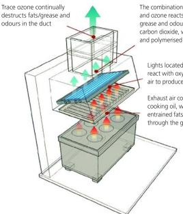
The combination of UV-C light and ozone reacts with the grease and odours to produce carbon dioxide, water vapour and polymerised grease (dust).
