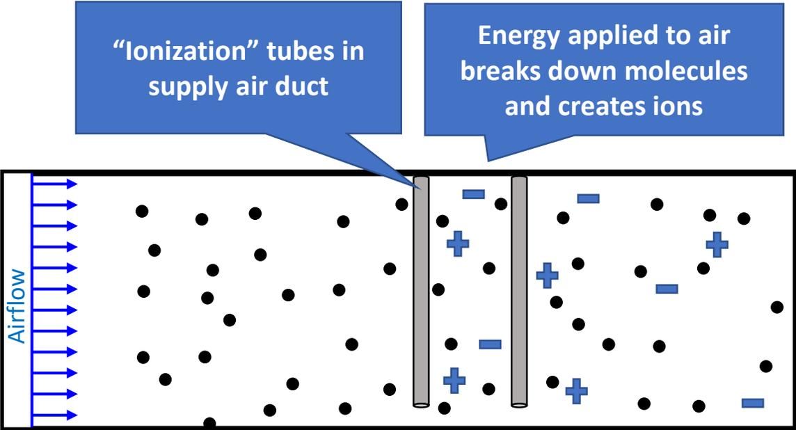
"Ionization" tubes in supply air duct
